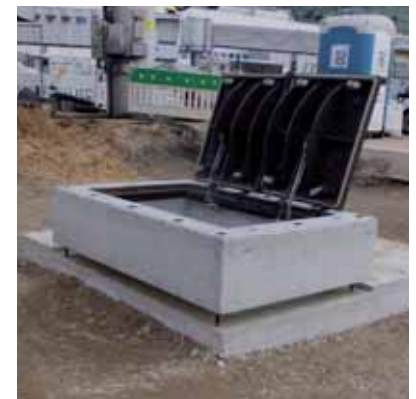
Kabelschachtafdekking druiwaterdicht, prefab in betonrand. Belastingklasse D400.
