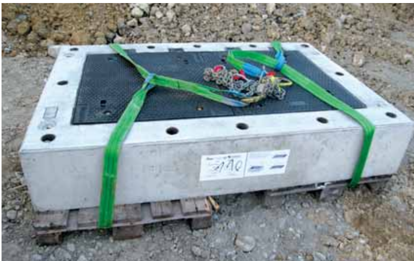
Kabelschachtafdekking druiwaterdicht, prefab in betonrand. Belastingklasse D400.
